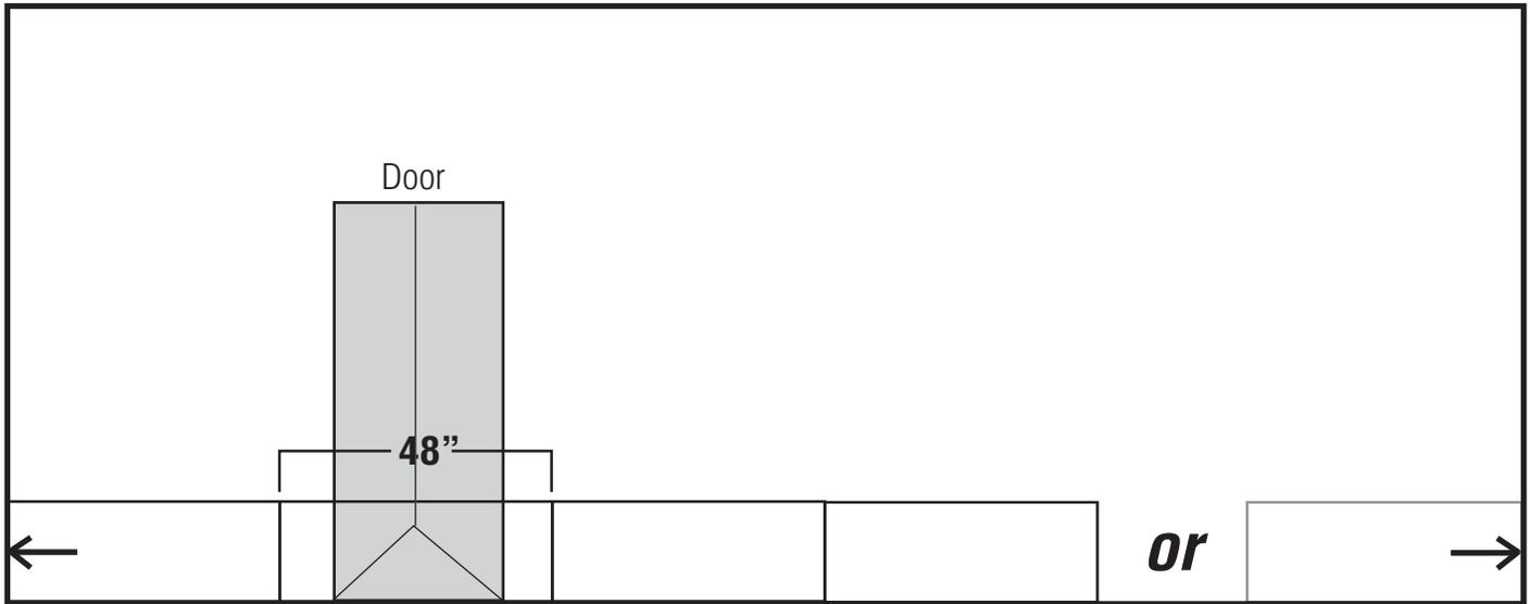
For the first course, you can start installing Strips from either gable end, or from any convenient point in the middle of the roof. You don't need to start at edge of the roof.
