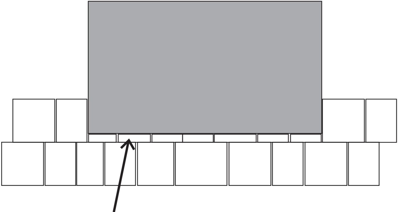
**Avoid** alignments that require attaching small sections of shakes below dormers or chimneys, or at the ridge.
