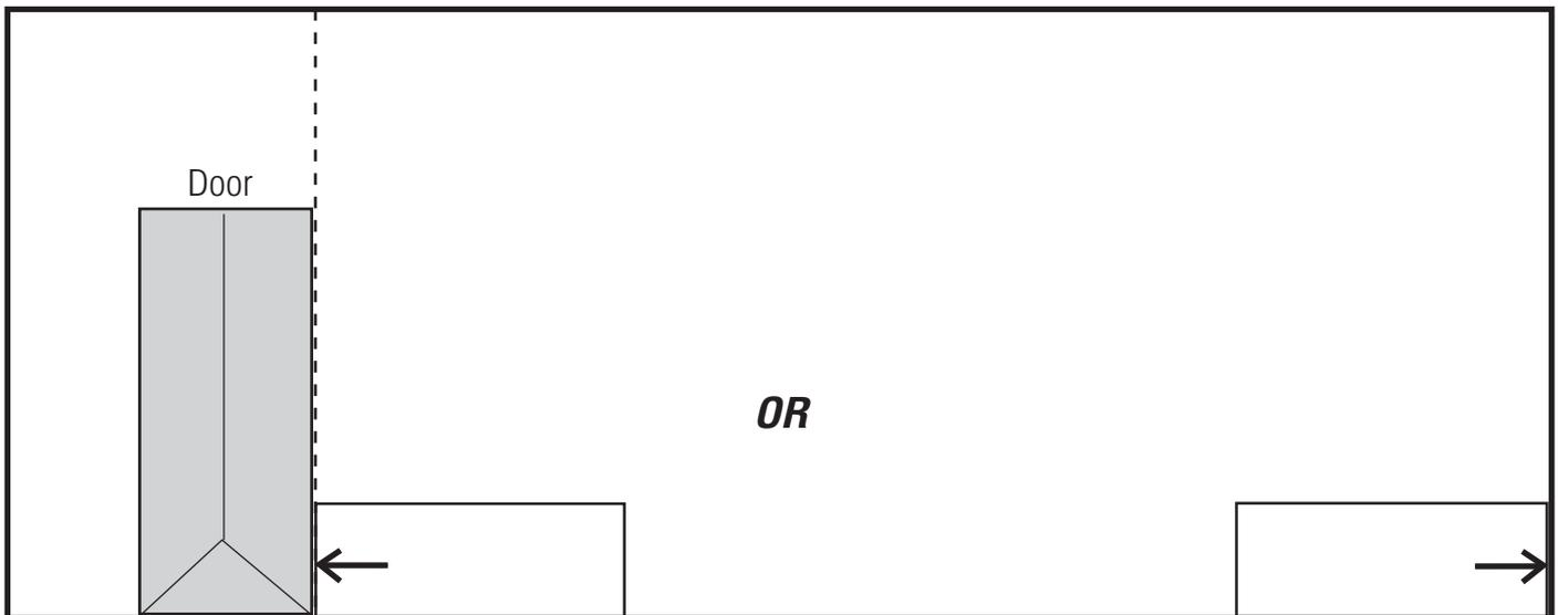
Install the first course allowing a 1/4" gap between Shake-Strips. Its 48" from any point on one Shake-Strip to the same point on the next. Double the first course as shown. Use the guide marks to offset the joints between the top and bottom courses, just as you will for adjacent courses.
