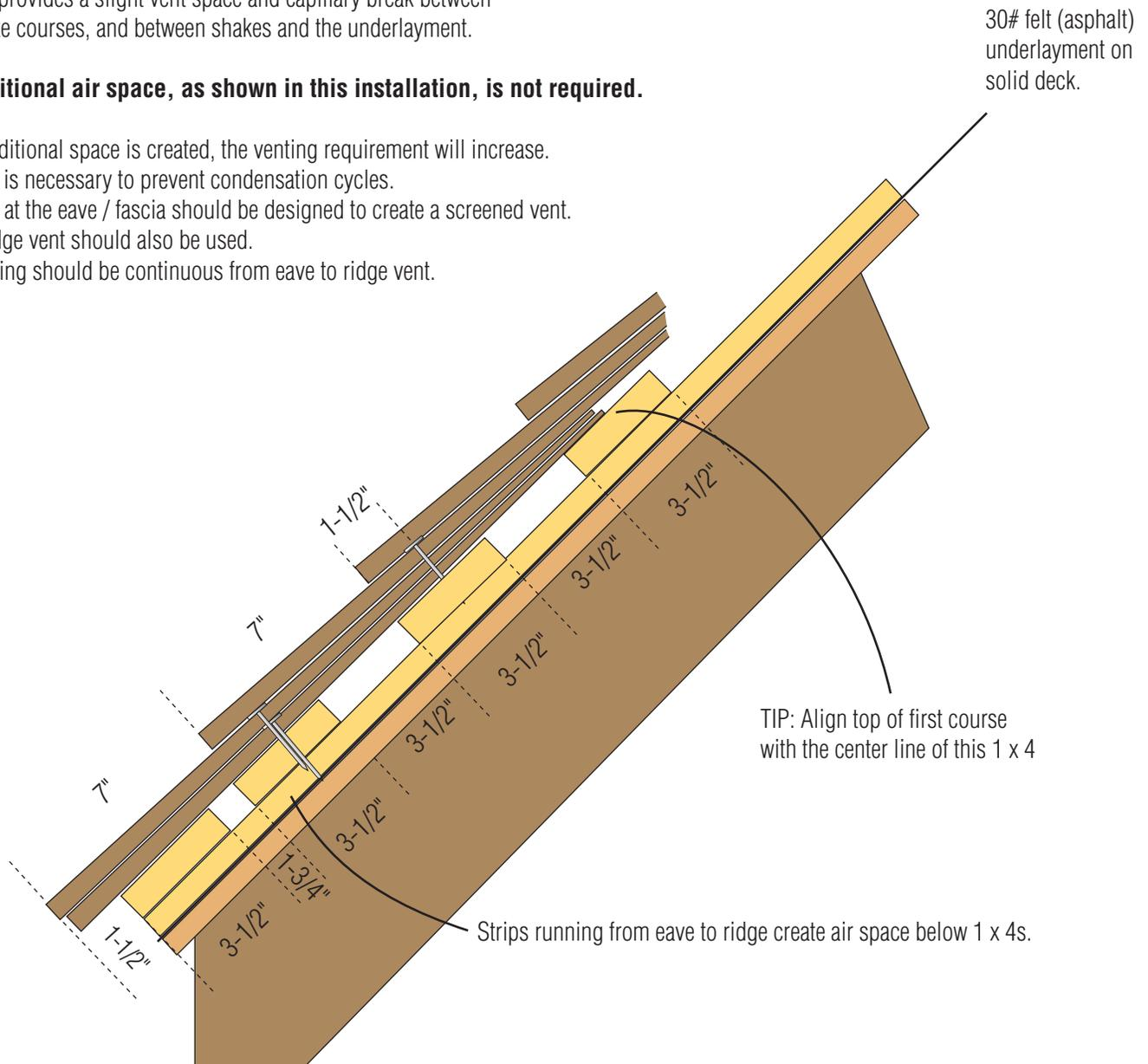
Trim at eave should be designed to allow airspace to be vented from eave to ridge vent.
